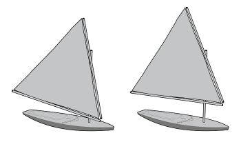
Place three wraps of electrical tape around the upper boom in the location where you will secure the halyard. This will prevent the halyard from slipping up to the next sail ring.
