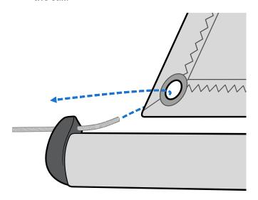
Feed the line back through the boom end cap and through the grommet again, so that the line is tripled.
