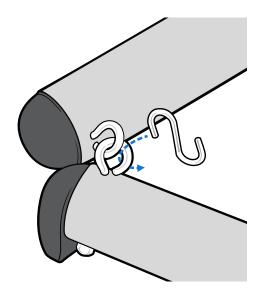
Loop the other end of the S-hook through the grommet in the tack of the sail (the corner of the sail where the two booms meet).
