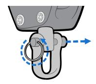
Locate the forward-most eyestrap attached to the lower boom and loop the shackle through it so that the ends with the holes are pointed away from the boom.
