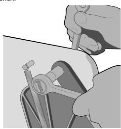
Note: The nut should be screwed on far enough for at least one thread to travel completely through the lock, but not so tight that you can not rotate the tiller up and down on the rudder.
