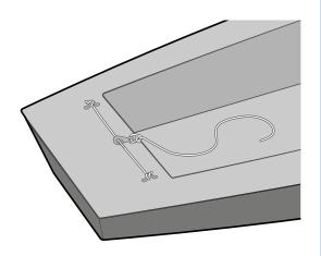
Feed the free end of the mainsheet through the two boom blocks, starting with the one closest to the stern (back of the boat), and bring the line down toward the mainsheet ratchet block.
