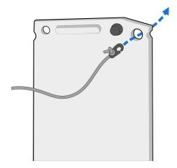
Lead one end of the shock cord around the mast and through the bow handle and back until you connect the two brummel hooks.
