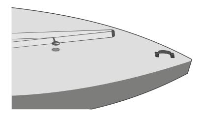
Hold the free end of the halyard, lift up the mast, and slide the base down through the gooseneck ring and into the mast step. Do not drop the mast into the tube to avoid damaging the mast step.
