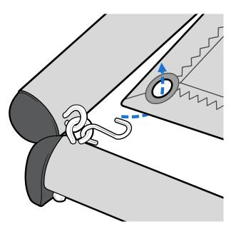
Using a pair of pliers, crimp the S-hook closed.
