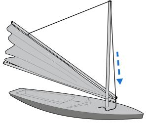
If the sail is not going up, you may need to lift the lower boom near the gooseneck with one hand while pulling on the halyard.
