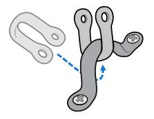
Align the hole in the bottom of the boom block with the holes in the ends of the shackle.
