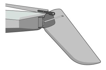
Leave the rudder in the kicked up (raised) position before launching.
