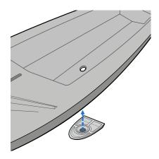
From the top (inside the cockpit), thread the bailer cap down through the cockpit hole and into the bailer housing. Screw the cap in place until it is hand tight.
