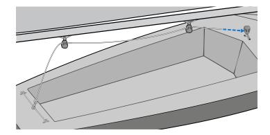
Note: The mainsheet ratchet block should only turn in one direction and make a ratchet or clicking sound. If turning the wheel does not make a sound, locate the lever and switch it to the ratchet position.
