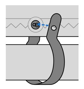
Note: The sail rings will be difficult to close. Pliers can be used to close the sail rings; however, be careful not to scratch the boom.
