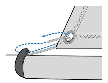
Secure by tying two half hitches around the lines. The outhaul line should be fairly snug.
