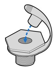
Locate the bailer opening on the underside of the hull. Place the bailer housing under the hull, with the ball and flat side facing toward the stern (back of the boat).
