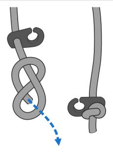
Thread one of the brummel hooks through the largest hole in the daggerboard.
