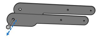
Slide the rudder between the tiller straps on the end of the tiller. Align the notches on the tiller straps with the notches on the rudder cheek and the holes in the tiller straps with the hole in the rudder.
