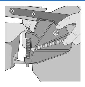
Release the pin, and the rudder should now be securely attached to the boat.
