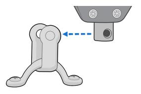
Insert the pin through all the aligned holes and secure it by threading the ring back through the small hole in the end of the pin.
