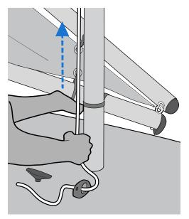
Continue pulling on the halyard until the clove hitch used to secure the halyard to the upper boom is right against the top of the mast.
